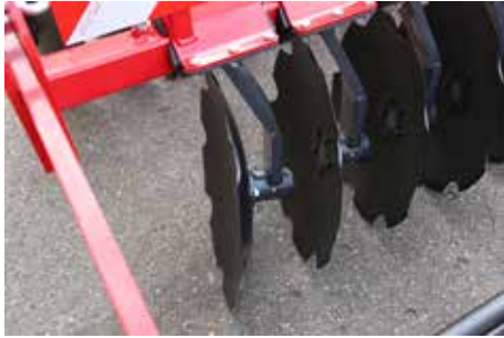
Torsion bar suspension for the discs
